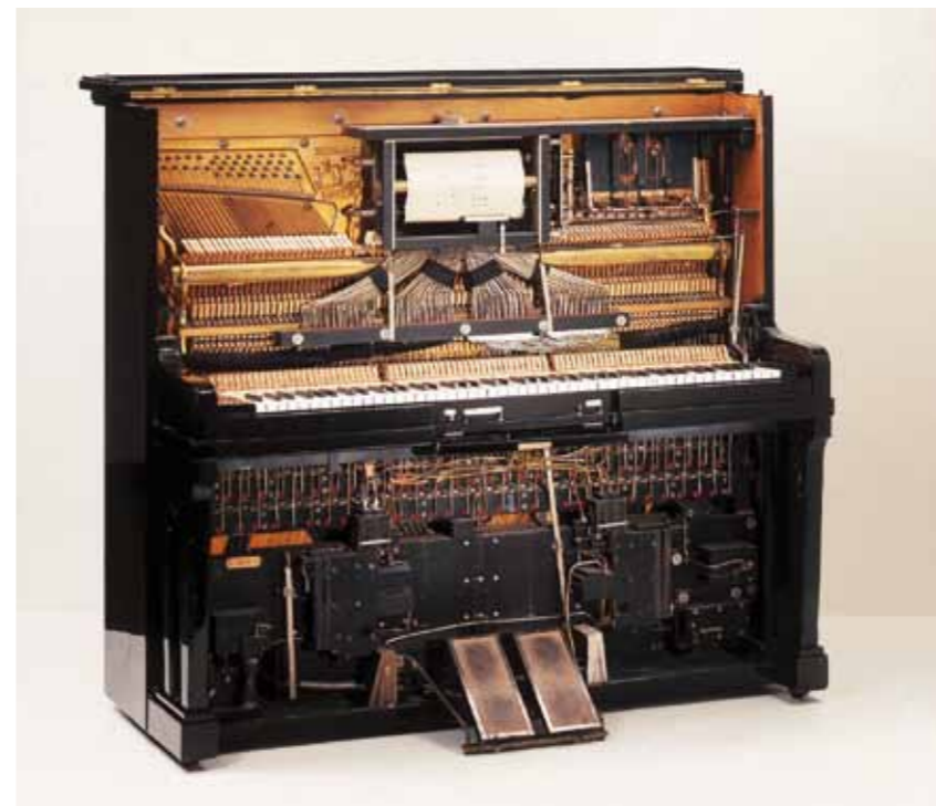
Schimmel player piano from the year 1920. The player mechanism was controlled by holes punched in a paper music roll – as found in the later IBM Hollerith machines.
