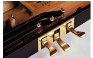
The muffer rail (céleste) is standard equipment in most Schimmel uprights. Depressing the practice pedal (middle pedal) causes felt strips to be lowered between the hammers and the strings, reducing the force of the hammer blow and, in turn, the volume of sound. Additionally, Schimmel offers the Schimmel TWINTONE Piano, wherein the middle pedal silences the hammer action, so no acoustic sound is generated and that of a digital piano can be heard through headphones or loudspeakers (see page 85).
