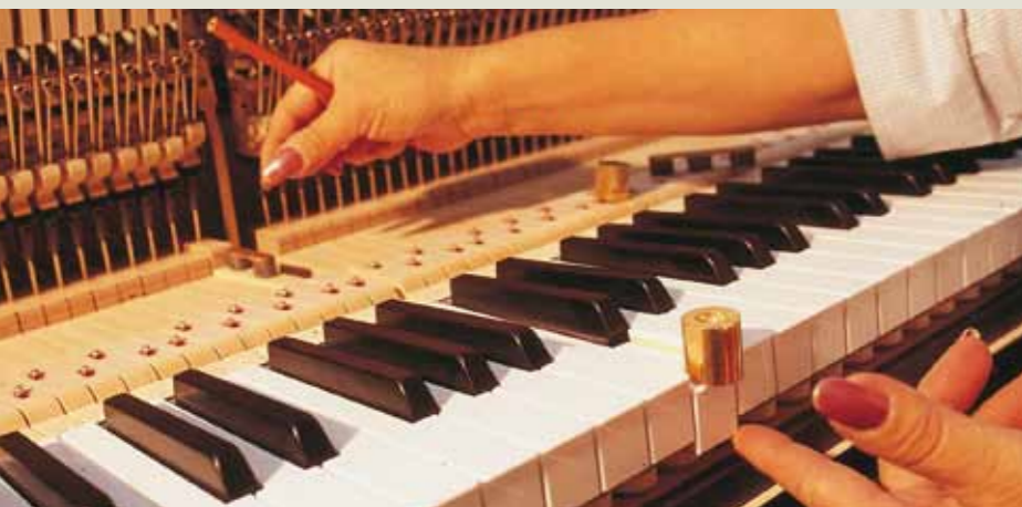
Each individual key is, of course, carefully balanced. In the photo we see a test weight on the front half of the key and two key leads which will later be inserted into it's the back half.
