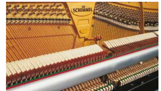
The muffer rail (céleste) is standard equipment in most Schimmel uprights. Depressing the practice pedal (middle pedal) causes felt strips to be lowered between the hammers and the strings, reducing the force of the hammer blow and, in turn, the volume of sound. Additionally, Schimmel offers the Schimmel TWINTONE Piano, wherein the middle pedal silences the hammer action, so no acoustic sound is generated and that of a digital piano can be heard through headphones or loudspeakers (see page 85).
