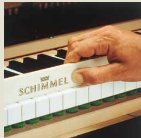
All keys must be perfectly leveled (above) and the key dip exactly to specification (left).
