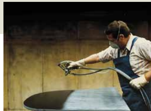
Applying a coat of black polyester lacquer
