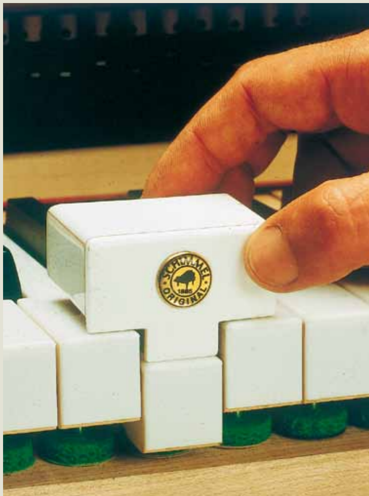
All keys must be perfectly leveled (above) and the key dip exactly to specification (left).
