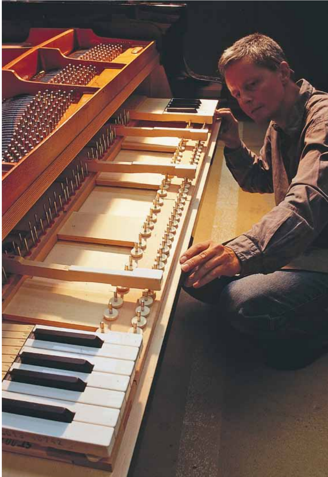
The keyframe must rest uniformly on the keybed, with no spaces in between. This requires skill and a sure eye.
