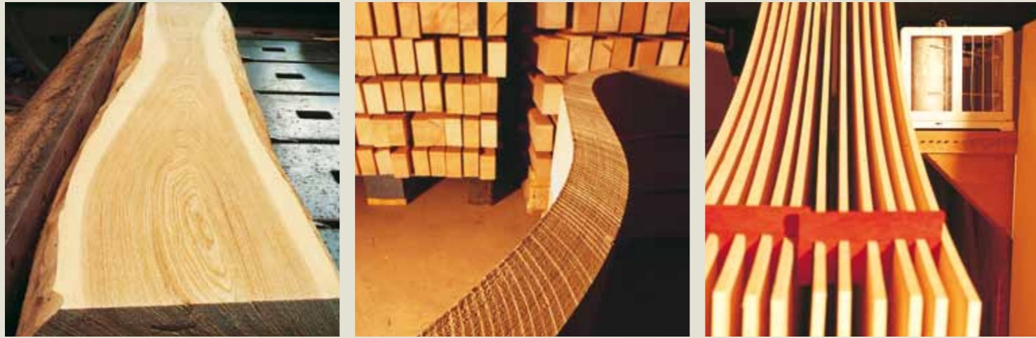
The seasoning (air drying) of solid-wood stock is as important for its long-term retention of value as its climatization following kiln drying.
