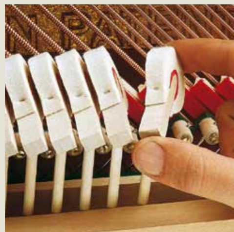
The gluing and alignment of hammers (left).
